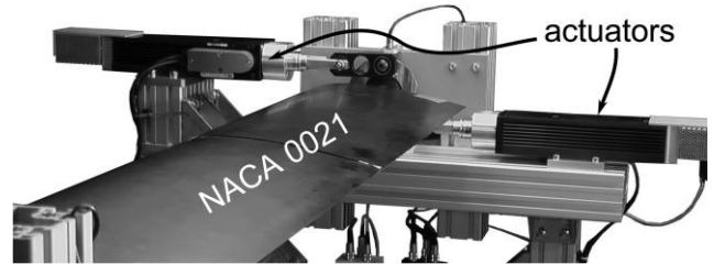
Figure 14. Motion apparatus used for the vortex generator airfoil
