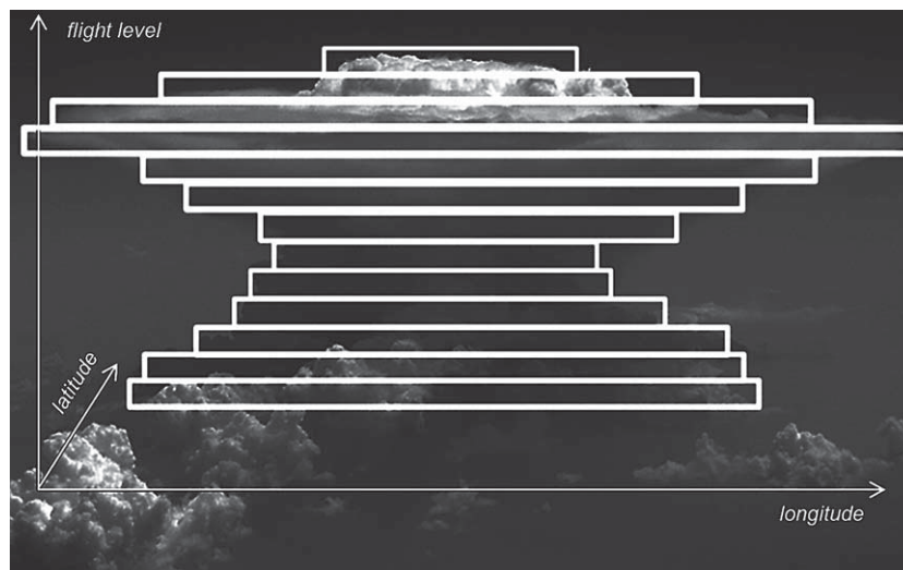
Fig. 2. A cumulonimbus cloud is considered as composed of horizontal layers at the various flight levels with different spatial extent.
